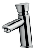
UTS 700 Self Closing Basin Tap • 2-4 litres per min flow rate • 3 seconds flow duration • 0.5-6.0 bar pressure range
