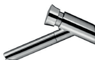
UTS 703L Self Closing Bib Tap • 2-4 litres per min flow rate • 3 seconds flow duration • 0.5-6.0 bar pressure range
