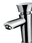
UTS 705 Self Closing Basin Tap • 2-4 litres per min flow rate • 3 seconds flow duration • 0.5-6.0 bar pressure range
