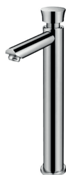
UTS 701 Self Closing Tower Basin Tap • 2-4 litres per min flow rate • 3 seconds flow duration • 0.5-6.0 bar pressure range
